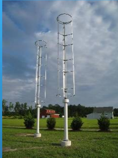
Residential wind turbines
